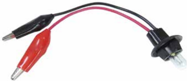
1.6. An auxiliary lamp for testing regulators, flasher relays and others (LA01):
