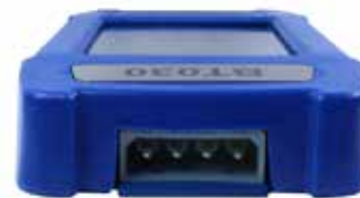
Fig. 2. Connector for diagnostic cable.
